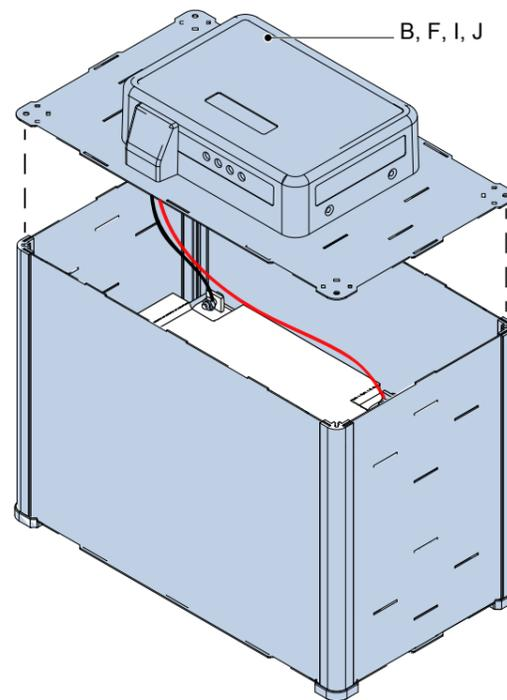
Fix the top plate by screwing four screws inside the profiles. Snap-in four corner-caps on top of each screw head.
