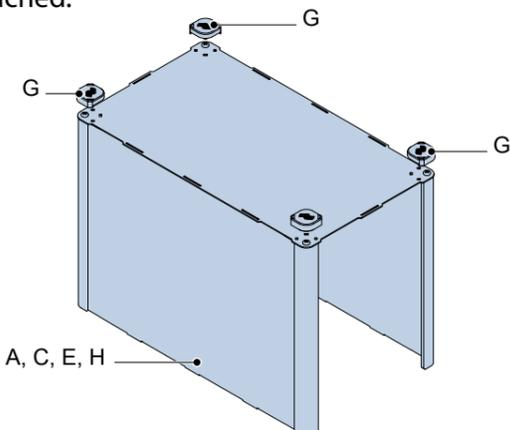
Carefully, lift the battery and slide it inside the enclosure from the top.
