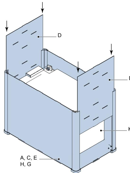
Fix the SHS-200 top-plate of the battery box. Use the 4 screws supplied together with the SHS wall-mounts.
