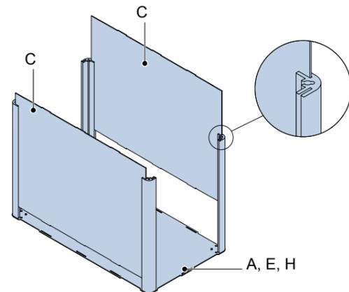
Snap-in four Corner-Caps on top of each screw head. The cap should click once it's properly attached.
