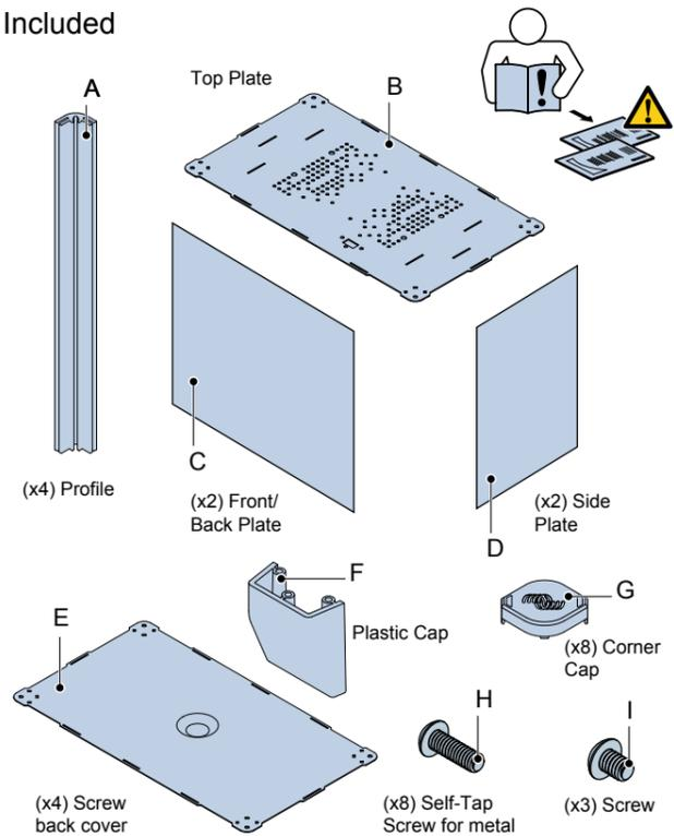
Slide the front and back plate through the profiles gap.
